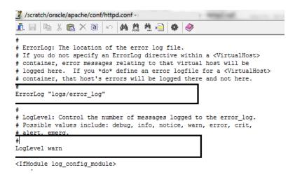
2. To enable debugging for communication between apache and weblogic add the following directives under Location tag
